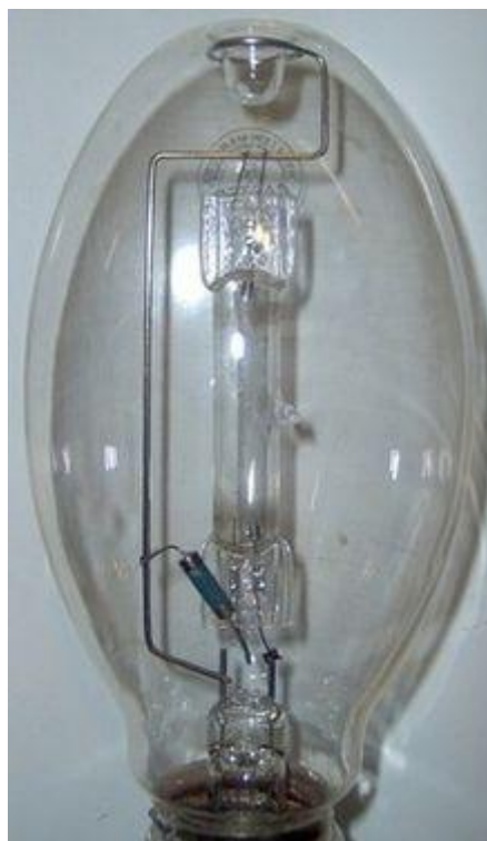
175W Mercury lamp, the small diagonal cylinder at the bottom of the arc tube is a resistor which supplies current to the starter electrode.
